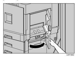
Move the blue lever up and down to feed the misfed paper, and then slowly pull out the paper.
