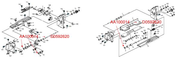
2. One 0454006Q will be replaced by B2342390. This will be replaced on B8332576 (Paper Feed Sensor Bracket).
