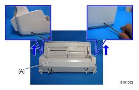
2. Release 2 snap points with the small minus screw driver. After that, lift up the top cover and remove it (Snapping points x 2).
