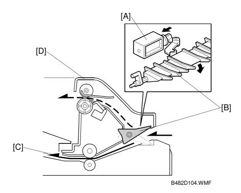
The junction gate [B] directs any paper reaching the bridge unit to either the upper tray (on top of the bridge unit) or to the finisher, depending on which has been selected.
