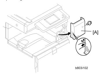
2. Remove the front right cover [A] (  $\mbox{\ensuremath{\beta}} \times 1$  ).
