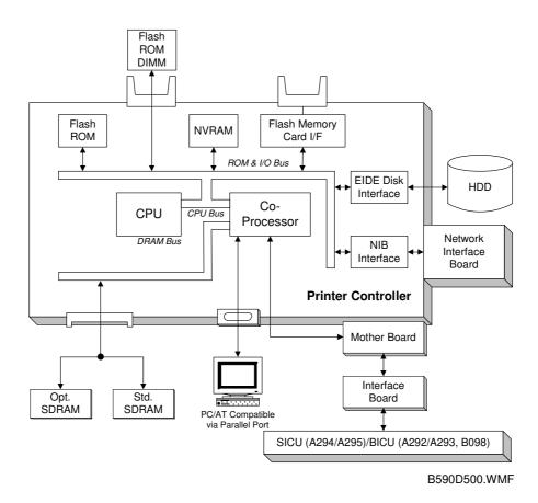
The above block diagram shows the major components of the printer controller. The main features of the controller are as follows.
