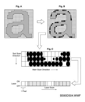
Usually, binary picture processing generates jagged edge on characters (Fig. A). The FCI reduces the edges of characters using edge smoothing.
