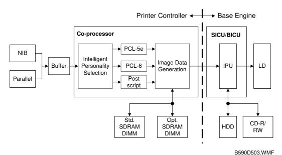
The printer controller receives print data from a PC through the parallel or network interface port. The co-processor handles the print data but it only makes raster image. All image processing, such as edge smoothing and toner saving, are done in the base engine.
