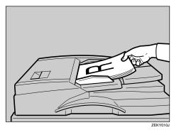
When set with this orientation, the original orientation setting for delivery must be changed.  $\Rightarrow$  P.48 "Original Orientation and Scan Area Setting"
