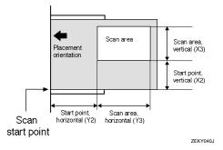
The maximum scan size is 432 mm in the Y direction (width) and 297 mm in the X direction (height). Keep the scan area settings within this range.
