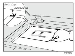
When set with this orientation, the original orientation setting for delivery must be changed. ⇒ P.48 "Original Orientation and Scan Area Setting"
