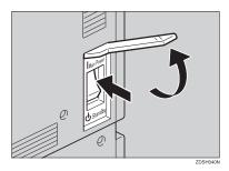
Turn on the operation switch. The On indicator should light.
