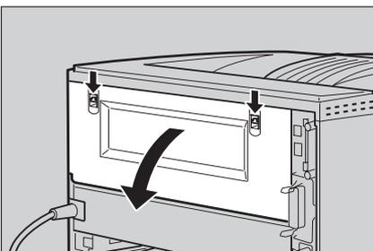
**5** Remove the rear cover in the horizontal direction.
