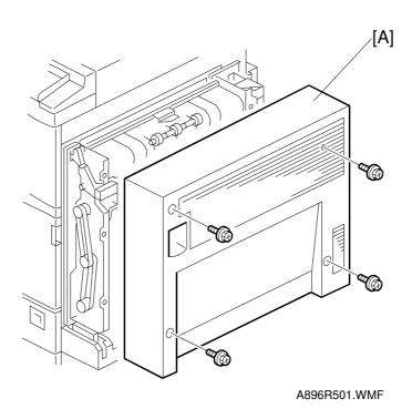
1. Remove the duplex unit cover [A] (4 screws).
