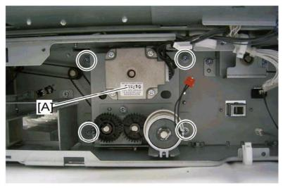
3. Inverter motor unit [A] ( x 4, u x 2)
