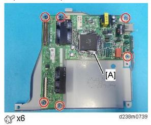
**<u>6.</u>** Remove the SG3 board [A] from one of the CCU I/F and SG3 board assemblies removed in step 5.
