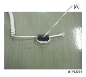
9. Connect the cable to the "TEL" jack on the left side of the controller box.
