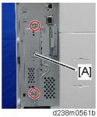
3. Remove the "TEL" [A] and "LINE1" [B] covers on the interface slot cover using a screwdriver.
