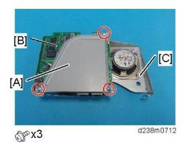
7. Insert the FCU [A] completely into the interface slot.
