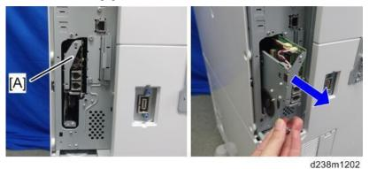
**<u>4.</u>** Switch the battery jumper switch [A] of the new fax unit to the "ON" position before installing.
