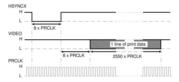
The FCU drops HSYNCX to low for eight PRCLK clock cycles before receiving each line of image data. Then, after the next eight cycles of PRCLK has passed, the controller starts to transfer one line of image data. The frequency of the PRCLK clock is between 1.3 MHz and 1.96 MHz.
