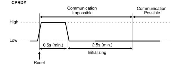
When the user resets the printer using function 35, the controller activates CPRDY for at least 0.5 s, then the controller initializes itself and the printing process is canceled. After initializing is completed, the controller will be ready to communicate with the host PC(s) and the FCU.
