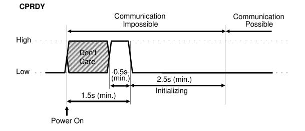
When the power is switched on, the controller raises CPRDY to high for at least 0.5 s, then initializes itself within 2.5 s. After initializing is completed, the controller will be ready to communicate with the host PC(s) and the FCU.
