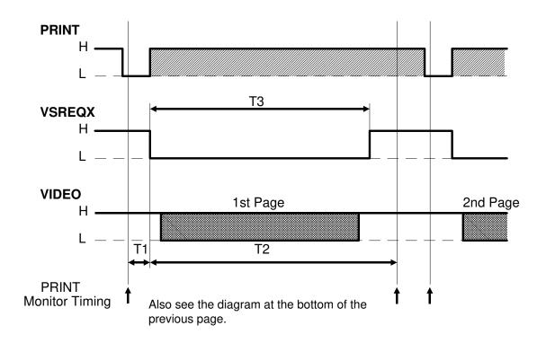
The FCU monitors the PRINT signal from the controller every 2 ms to detect if a print request is coming from the controller or not. After T1 has passed since the FCU detected the PRINT signal to be active (low), the FCU drops VSREQX to low so that the controller can acknowledge that the printer is ready to receive one page of image data. After one page of data has been received from the controller, the FCU inactivates the VSREQX signal until PRINT is activated again for printing the next page.
