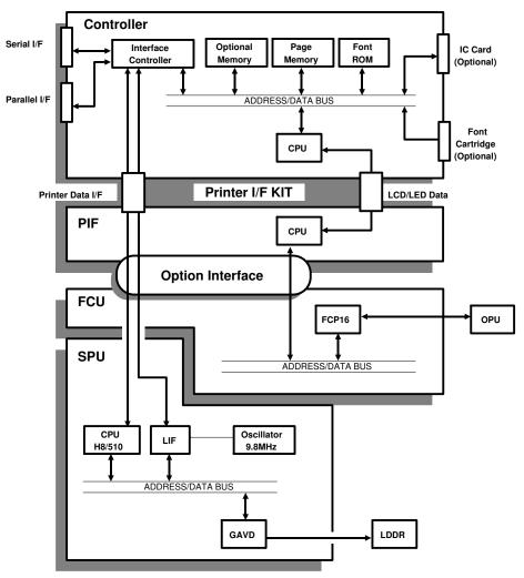
The printer interface kit consists of two PCBs: the printer controller board (Controller) and the printer interface board (PIF).
