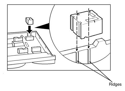
**Note:** To prevent the spacer from being out of position, ridges have been added to the rear fence of the cassette body as shown at the same time. However, its part number (P/N AF011102) has not been changed. It is recommended to use two-sided tape to secure the spacer when it is used for the old cassette body.
