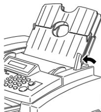
**2** Open the front paper feed unit by moving it to forward.
