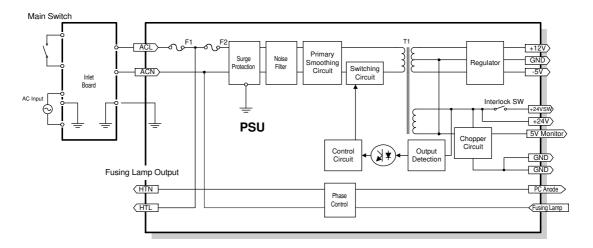
PSU:120V/230V The values of some parts on the primary side are different between the 120V and 230V versions.
