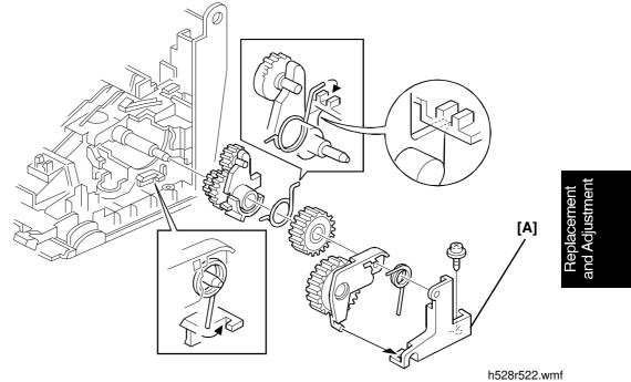
To remove components in the fusing section, remove the top cover assembly first (see Top Cover Assembly).
