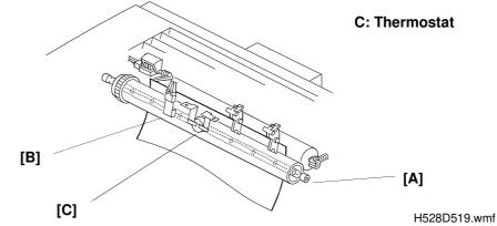
The power supplied to the lamp [A] is controlled by the MCB. The MCB uses the thermistor [B] to determine when to turn the fusing lamp on and off.
