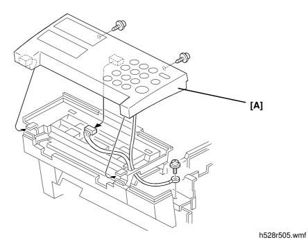
A: Operation Panel Assembly (2 screws, 1 tapping screw with ground wire, 1 connector, 2 hooks)
