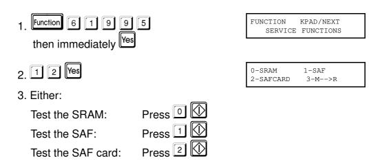
If test is successful, the display shows "OK". If test is unsuccessful, the display shows "ADDRESS=".
