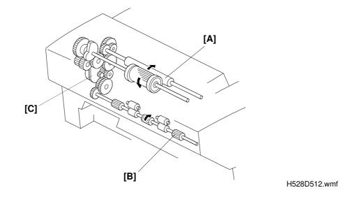
The document is fed into the scanner by the scanner roller [A], and fed out by the exit roller [B]. The tx motor [C] drives the scanner roller and the exit roller.
