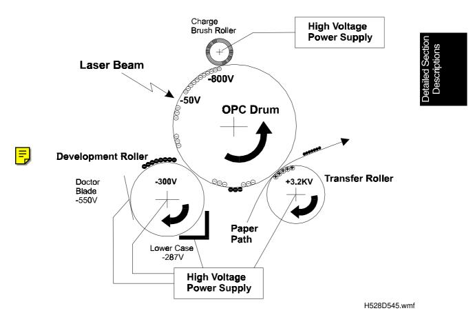
This machine uses a "write to black" system, using negative toner.
