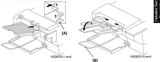
The document sensor [A] detects when a document is placed in the ADF. The fold-out extension [B] helps support longer documents.
