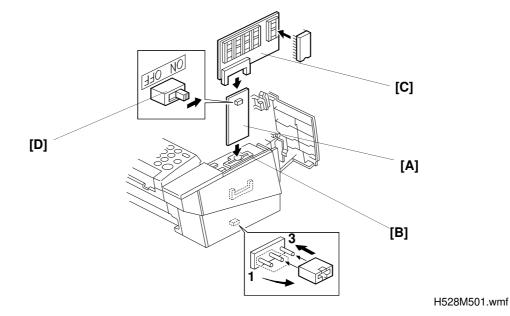
2. Insert the Flash/SRAM Copy Tool [A] into the IC card slot [B], then connect the EPROM board with new software [C] to the opposite side of the tool.
