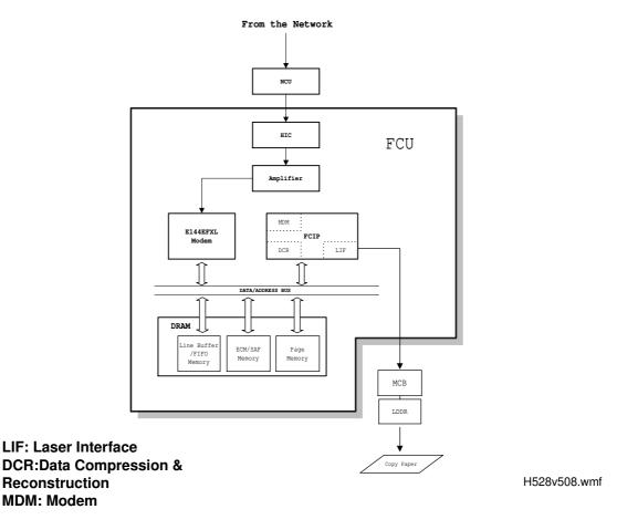
Data from the line passes to the modem through the NCU and hybrid IC. After the modem demodulates the data, the data passes to the DCR block, through either the FIFO or the ECM memory, where the data is decompressed to raster image data.
