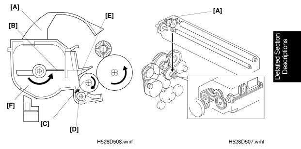
This machine contains a development toner magazine (DTM) [A], which contains the toner agitator [B], development roller [C], toner supply roller [D], doctor blade [E], and the toner tank [F].
