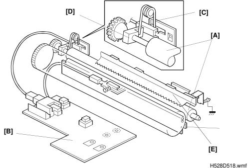
A transfer bias of +3.2 kV is applied to the transfer roller [A] from the high voltage supply [B]. This charge is applied through the torsion spring [C] and the conductive supporter [D].
