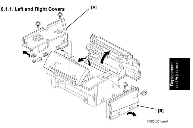
A: Left Cover (2 screws, 2 hooks) B: Right Cover (2 screws, 2 hooks)
