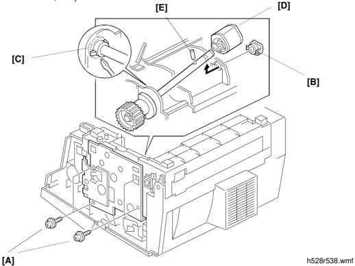
Remove 4 screws [A]. Remove bushing [B] (1 E-ring, 2 hooks). Unhook the two hooks on bushing [C]. Remove the pick-up roller [D] (1 pin).
