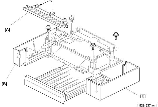
A: Upper Guard (3 hooks) B: Left Cover (2 screws, 2 pins) C: Right Cover (2 screws, 2 pins)
