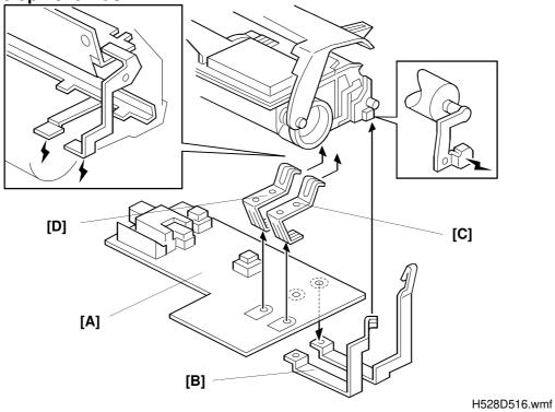
The high voltage power supply [A] applies different voltages to the components of the DTM. The applied voltages are:
