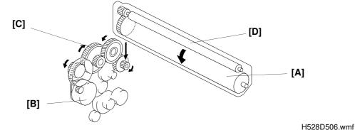
This machine uses an organic photoconductor drum [A]. The diameter of the drum is 30 mm. It is driven by the main motor [B] through a gear train [C]. The charge brush roller [D] is also driven by the main motor. The drum cartridge is replaceable by the user.
