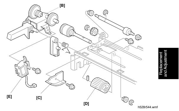
B: Feed Gear Assembly (1 screw, 1 screw with upper left feed guide [C])
