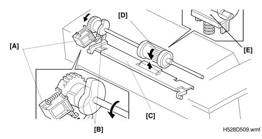
When the document pick-up solenoid [A] is turned on, it allows the tray lifting cam [B] to rotate. This allows the document plate [C] to be pushed up by a spring under the plate. The document pick-up roller [D] feeds the top sheet of the document into the scanner. The separation pad [E] prevents the document pick-up roller from feeding more than one sheet at the time.
