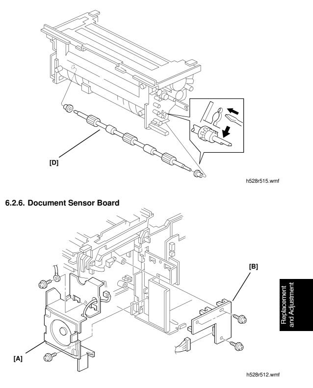
A: Speaker Mount Bracket (1 screw, 1 screw with ground wire, 1 connector) B: Document Sensor Board (3 tapping screws, 1 connector)
