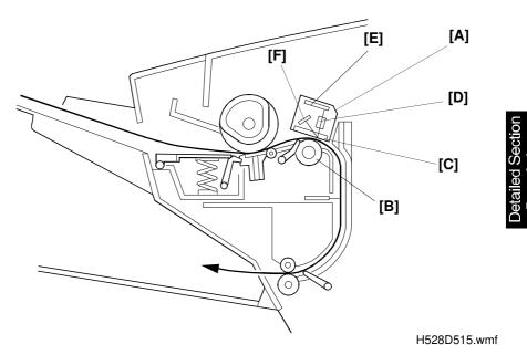
The scanner consists of a contact image sensor (CIS) assembly [A] and a scanner roller [B]. Inside the CIS are an exposure glass [C], a rod lens array [D], an image sensor [E], and an LED array [F].
