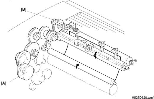
The main motor [A] drives the fusing unit through a gear train. The paper exit sensor [B] detects when the paper is fed out of the unit.
