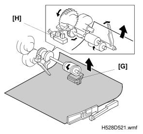
The paper activates the registration sensor [H]. This sensor warns the printer that a sheet of paper is coming, to initialize the laser engine. It is also used for paper size and jam detection. If the paper size is determined not to match the selected paper size, a paper size error is detected. The machine stops printing and indicates the user of the incorrect paper size, but the image data is retained and will be printed out when the paper is reset in the tray.
