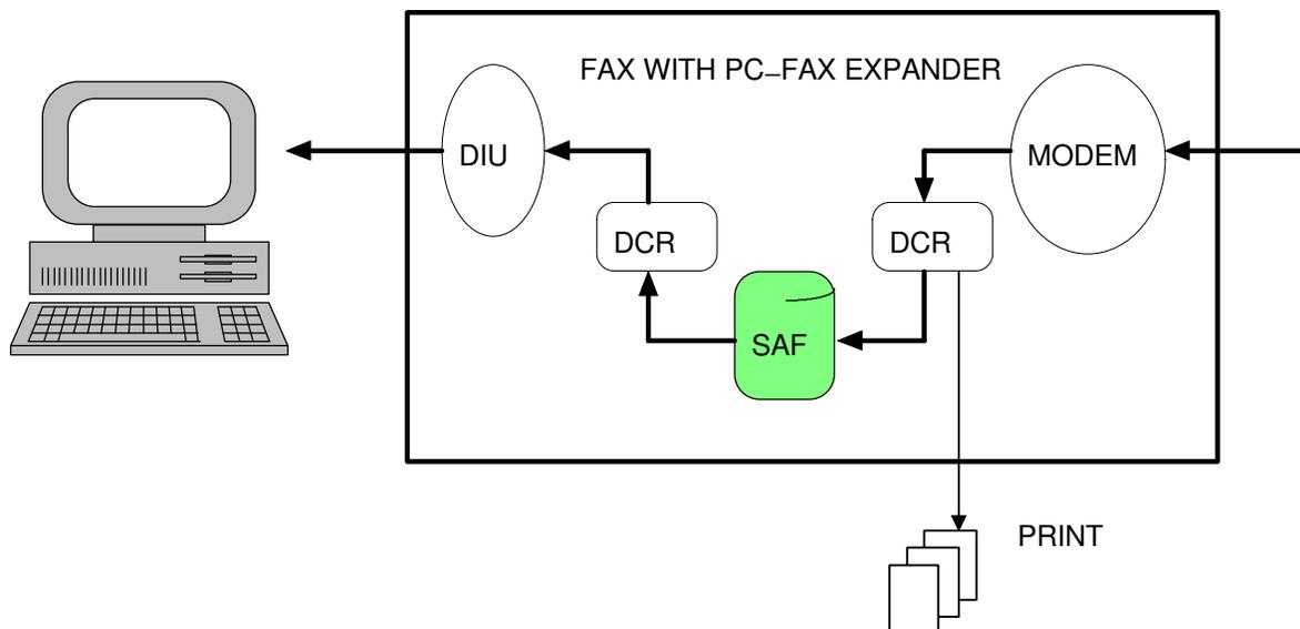
With Function 16, the fax machine will scan a document and send it to the PC, where it will be received by the faxing application.
