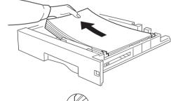
4. Adjust the paper fences to the paper size. To move a fence, pinch the top lever in and slide the fence in or out as shown. Make sure the positions of the two side fences match the paper size by checking them against the scale printed on the bottom of the feed unit. The fences should be aligned so that the inside edge of each fence is just touching the line of the scale.
