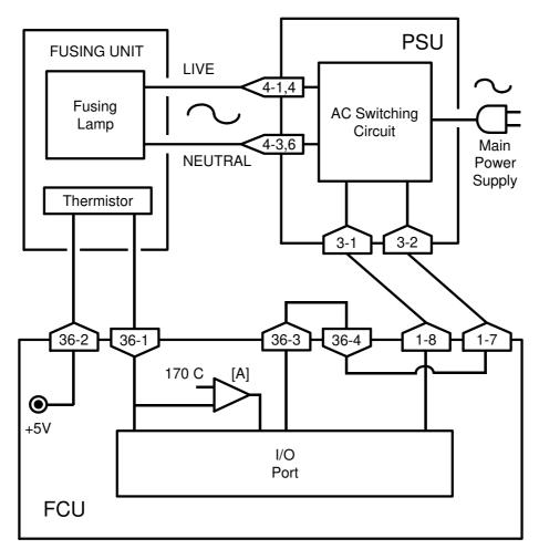
The circuit shown in the above diagram controls the fusing unit.
