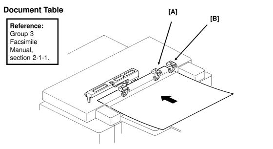
• The scanner is A3-width [11.7"], with a B4 document width detector [A] and an A3 document width sensor [B].
