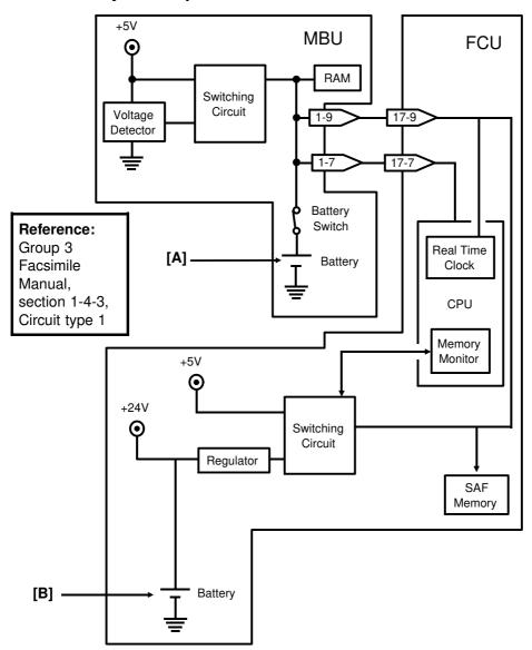
The battery [A] on the MBU backs up the RAM on the MBU, which contains system parameters. It also backs up the real time clock in the cpu. This battery is not rechargeable. CN1-7 tells the cpu whether the back-up power (CN1-9) comes from the battery or from the +5V power supply.
