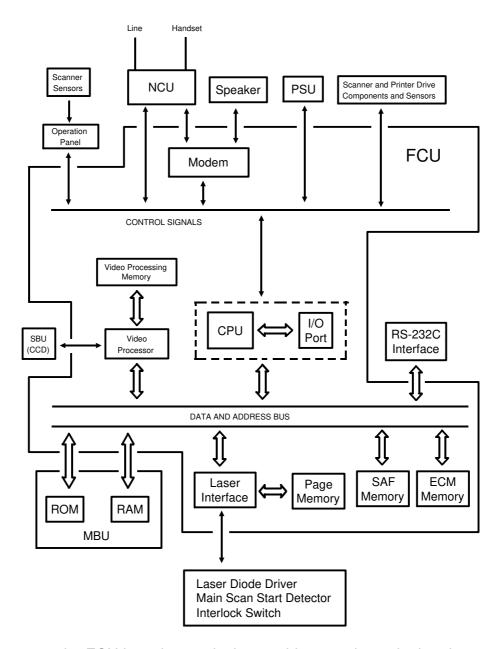
The cpu on the FCU board controls the machine, as shown in the above drawing. There is no modem board in the machine; the modem consists of a chip on the FCU board that carries out all the analog and digital functions of a fax modem.
