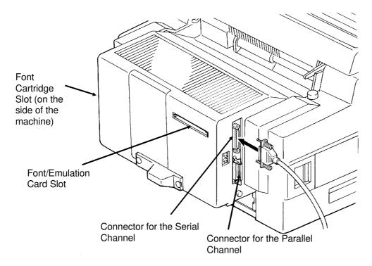
There is no cable provided with the printer interface kit. To connect the printer to your computer, you will need either:
