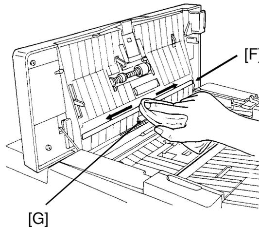
8. Clean the R1 and R2 rollers [H] with the soft damp cloth. To rotate the rollers, gently hold the cloth down on the rollers and turn the main power switch on. The rollers will rotate once. These rollers are near the ③ decal.
