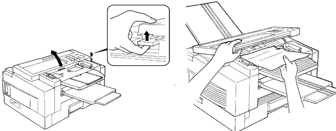
1. Pull up the scanner release and open the scanner.
