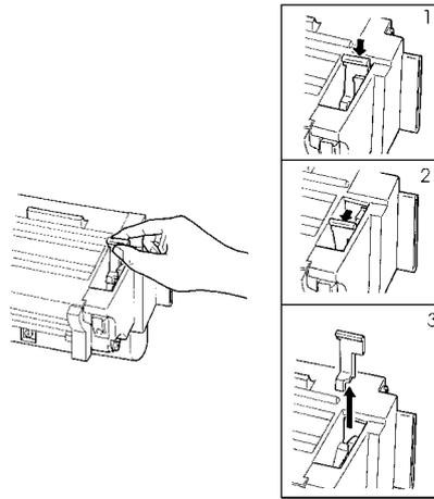
6. Slide the new toner cassette into the machine along the rails until it stops.
