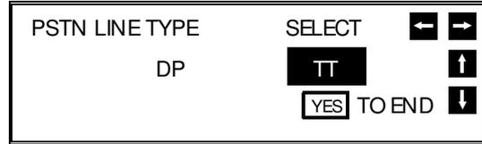
The first displayed item is the telephone line type: DP = Pulse Dial, TT = Touch Tone. In the above display, TT is currently selected.
