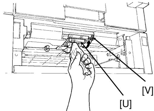
3. Clean the paper feed rollers [W] in the cassette with the soft damp cloth, while rotating them as shown in the diagram.
