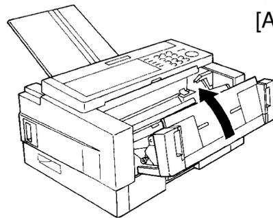
8. Put the tray and document table back, then switch the machine back on.
