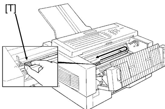
9. Remove the sheet of paper from the master belt, and put back the toner cassette.
