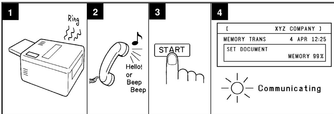
1. The machine rings continuously until you answer the call. Pick up the handset.
