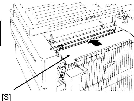
8. Slide the blue plastic corona wire cleaner [T] from its home position all the way across to the right side of the machine. Then move it back to the home position; you will hear a click when the cleaner reaches home position.
