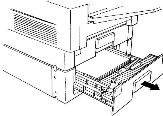
2. Clean the paper feed roller [U] with the soft damp cloth, while rotating it in the direction shown in the diagram.
