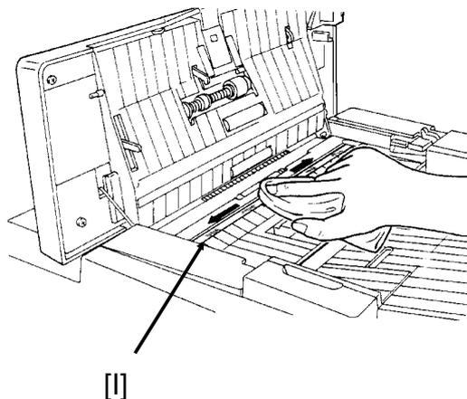
11. Clean the pick-up and feed rollers [J] with the soft damp cloth, while rotating the rollers in the direction shown in the diagram. These rollers are near the ② decal.
