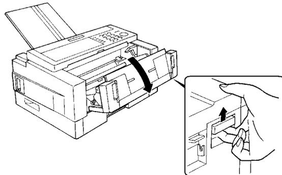
3. Pull out the jammed paper carefully by the leading or trailing edge, or by the center if both edges are jammed.
