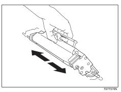
**1** Hold the cassette as shown and rest it in the machine. Make sure it fits in the slots provided on either side.
