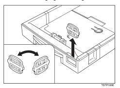
Replace the plate, orienting it so that the letter symbol is visible in the window at the front of the cassette.
