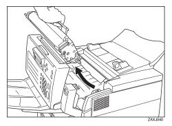
**B** Remove any jammed paper underneath.
