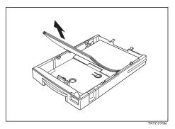
If this is the main cassette and the metal base plate is raised, push it firmly down until it locks into place.
