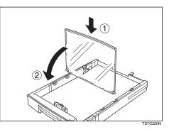
**E** Replace the cassette. Push it in firmly until it lock into place.
