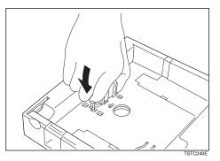
**2** Remove the side rail (Squeeze in one of the plastic tabs on the underside of the cassette to loosen it).
