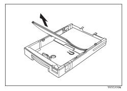
If the metal base plate is raised, push it firmly down until it locks into place.
