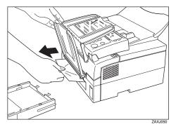
**B** Push down the paper so that the base plate locks into place.
