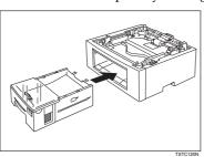
**6** Lay the machine on top of the unit as shown.
