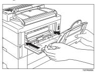
Before you use the Multi - purpose Feeder, you need to change the paper size setting to match the size of paper you will be using by function 37. See P.138 "Changing the Paper Size Settings"
