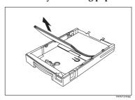
4 If this is the main cassette and the metal base plate is raised, push it firmly down until it locks into place.
