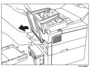
**2** Push down the paper so that the base plate locks into place.
