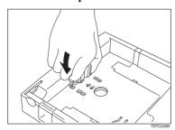
Remove the side rail (Squeeze in one of the plastic tabs on the underside of the cassette to loosen it).
