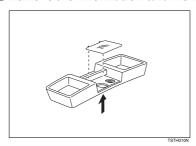
2 Attach the holder to the bracket with the two screws provided.
