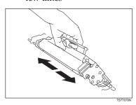
**E** Hold the cassette as shown and rest it in the machine. Make sure it fits in the slots provided on either side.
