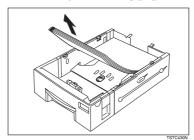
4 Squeeze the green end plate slightly and remove it.
