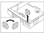
Replace the plate, orienting it so that the A4 symbol is visible in the window at the front of the cassette.
