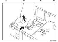
**5** Insert the end plate into the A4 slot as shown.
