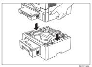
Make sure the machine and unit fit together correctly. If they are not aligned, the machine will not be able to detect the second cassette when you try and change the paper size setting with function 37. See P.138 "Changing the Paper Size Settings"
