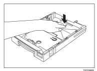
Squeeze the green end plate slightly and remove it.
