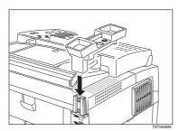
**5** Plug the handset jack into the "TEL1" socket at the rear of the machine.
