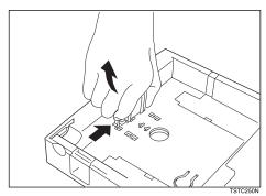
1 Insert the end plate into the A4 slot as shown.
