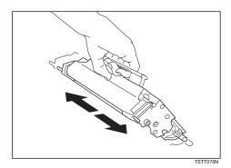
16 Hold the cassette as shown and rest it in the machine. Make sure it fits in the slots provided on either side.
