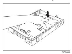
**5** Squeeze the green end plate slightly and remove it.
