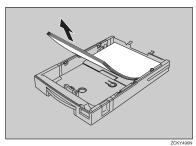
If the metal base plate is raised, push it firmly down until it locks into place.
