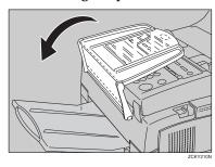
4 Push down on the paper until you hear the base plate lock into place.
