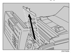
Install the cleaning pad a shown in the illustration.
