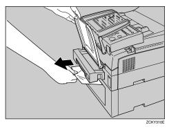
☐ Remove any paper that may have dropped inside the machine in the area vacated by the paper cassette.
