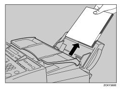
Remove the bypass feeder.
