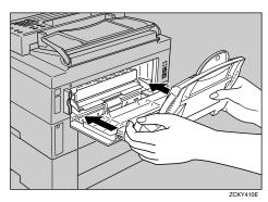
Square the edges of the paper and load it face down into the feeder.
