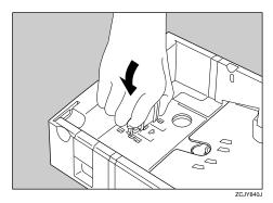
A Remove the side rail. (Squeeze in one of the plastic tabs on the underside of the cassette to loosen it.)
