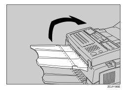
13 Hold up the print delivery tray and remove any jammed paper.
