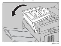
Push down on the paper until you hear the base plate lock into place.
