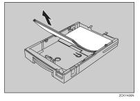
4 If the metal base plate is raised, push it firmly down until it locks into place.
