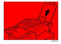
**2** Lift up the tabs located on the sides of the machine and open the front unit.
