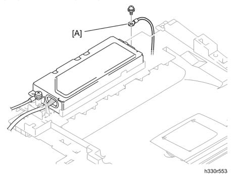
2. Remove the NCU FG harness ASSY [A] (  $\mbox{\it P}$  x 1; pan (S/P washer) M3.5x6).
