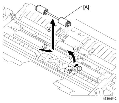
14. Release the hook to remove the pressure roller ASSY [A].
