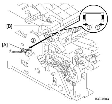
2. Release the two hooks and remove the new toner sensor harness ASSY [A] from the main frame L [B].
