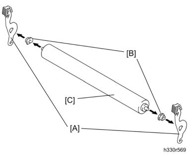
6. Remove the two PR arm ASSYs [A] and two PR bushes [B] from the pressure roller [C].
