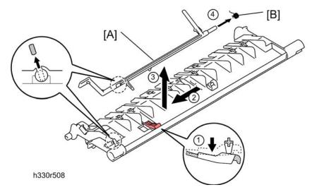
3. Remove the paper eject actuator [A] and the eject actuator spring [B].
