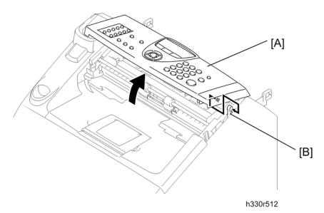
2. Open the panel unit [A] and remove the link stopper [B].
