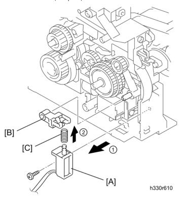
2. Remove the P/R solenoid ASSY [A], the P/R solenoid lever [B] and the solenoid release spring P/R [C] ( $P \times 1$ ; B M3×10).
