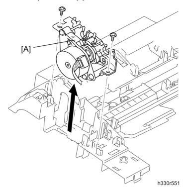
27. Remove the scanning driver ASSY [A] (  $\mathscr{F}$  x 2; B M3x8).
