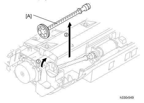
25. Remove the LF roller gear [A].
