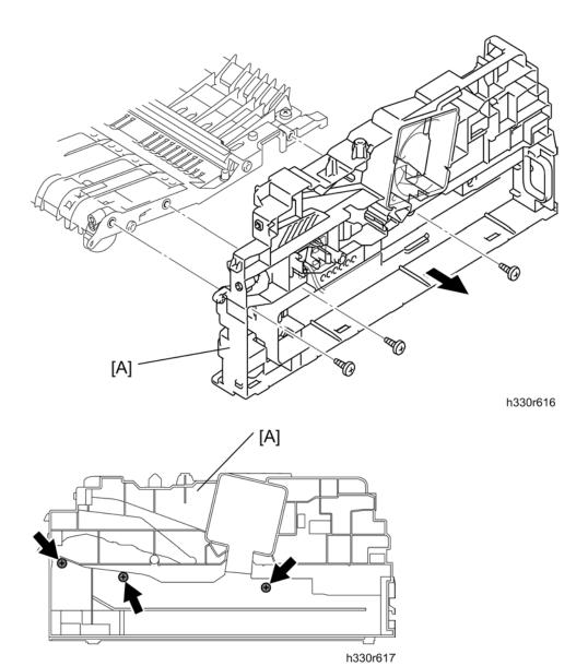
2. Remove the main frame R [A] (  $\Re$  x 3; B M4x12).
