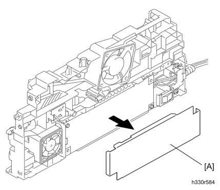
5. Remove the LV insulation sheet [A].
