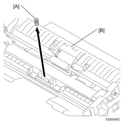
16. Remove the LF spring [A] from the top cover [B].
