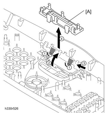
12. Release the two hooks to remove the back light holder [A].
