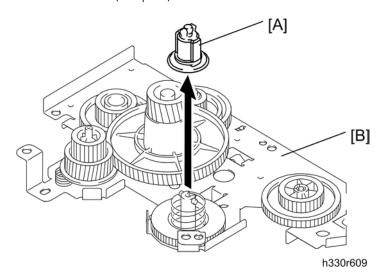
2. Remove the develop joint [A] from the gear plate calking ASSY [B].
