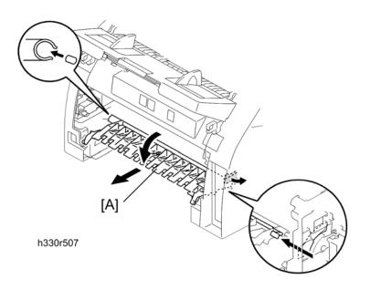
2. Remove the rear chute cover [A].
