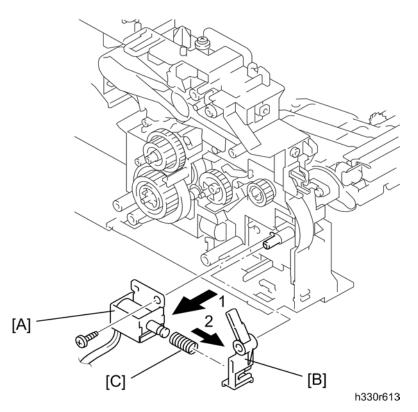
3. Remove the F/R solenoid ASSY [A], the F/R solenoid lever [B] and the solenoid release spring F/R [C] ( $\mathscr{F} \times 1$ ; B M3×10).
