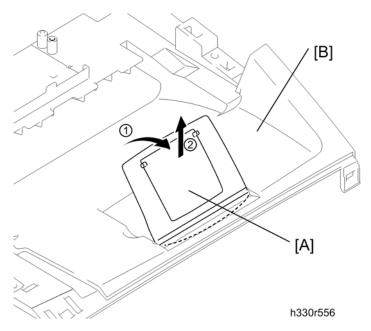
1. Remove the paper stopper ASSY [A] from the inner chute cover ASSY [B].
