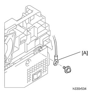
5. Remove the the NCU FG harness ASSY [A] (  $\mathscr{F}$  x 1; pan (S/P washer) M3.5x6).
