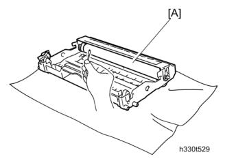
3. Wipe the surface of the exposure drum [A] with a cotton swab until the dust or paper powder on the surface comes off.
