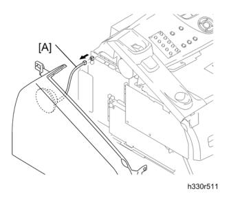
4. Disconnect the connector [A] of the speaker ASSY.
