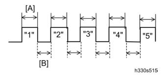
These selectors set the tone signal transmission time length [A] and minimum pause [B] in tone dialing. (Example: If "1," "2," "3," "4," and "5" are dialed.)
