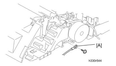
19. Remove the scanning drive LF FG harness ASSY [A] ( x 1; B M3x4).
