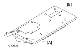
Is the scanner interlock lever [A] damaged? Is the scanner mirror broken or loose?
