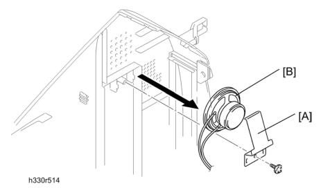
2. Remove the speaker hold spring [A] and speaker ASSY [B] (  $\mathscr{F}$  x 1; B M3x8).
