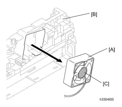
4. Release the harness from the hook, and then remove the fan motor 60 unit [A] from the main frame R [B].
