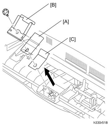
4. Remove the separation rubber [A], ADF plate spring [B] and front plate spring [C] ( x 1; B M3x6).
