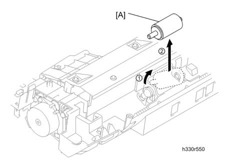
26. Remove the separation roller [A].
