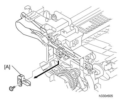
2. Remove the toner sensor PCB ASSY [A] (  $\slash\hspace{-0.4em}P \times$  1; B M3x6).
