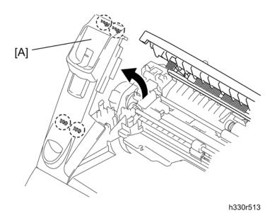
3. Release the four hooks to remove the handset holder [A].
