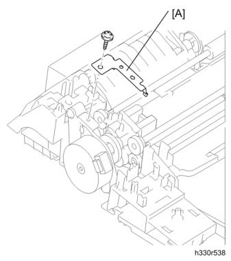
11. Remove the LF ground plate [A] ( $\mathscr{F}$  x 1; S M3x6).
