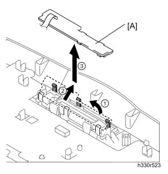
9. Release the three hooks to remove the panel PCB ASSY [A].
