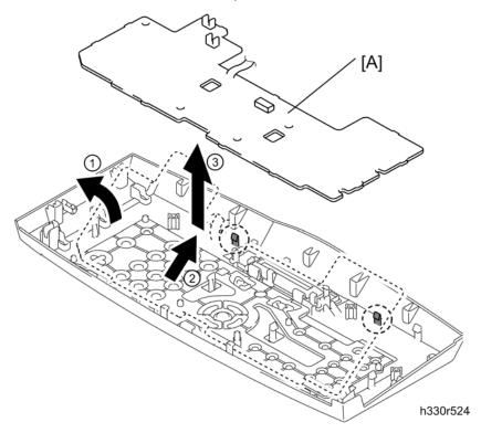
10. Release the two hooks to remove the panel PCB ASSY [A].
