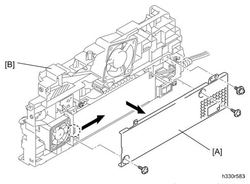
4. Remove the LV shield plate cover [A] from the main frame R [B] ( x 2; S M3x6, x 1; pan (S/P washer) M3.5x6).
