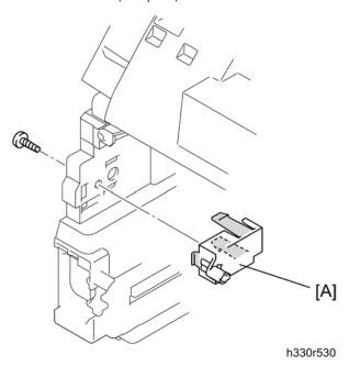
2. Remove the rear cover stopper [A] (  $\slash\hspace{-0.6em}P \times 1; \ B \ M4x12).$
