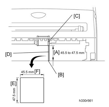
Check that the distance [A] between the floor [B] and the separation roller collar [C] of the pickup roller holder ASSY is 45.5 to 47.5mm by using the plate jig [D]. If not, re-assemble the chute base.
