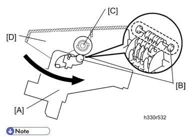
• Re-assemble the inner chute [A] while pushing onto the pinch roller [B] of the inner chute with the eject roller [C] of the top cover [D].
