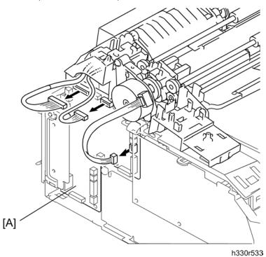
4. Disconnect the three connectors from the main PCB [A].
