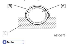
• When re-assembling the heat roller [A], assemble the HR bush [B] onto the fuser frame [C] referring to the figure above.
