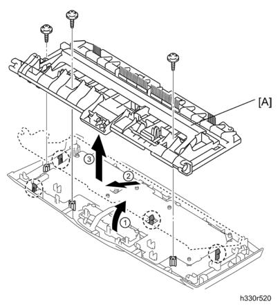
6. Release the four hooks to remove the panel rear cover [A] ( $\mathscr{F}$  x 3; B M3x8).
