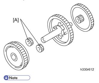
• The gear ASSY contains the small gears [A]. Be careful not to lose them by disassembling the gear ASSY.
