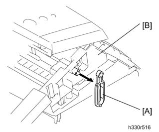
3. Remove the link stopper [A] from the top cover [B].
