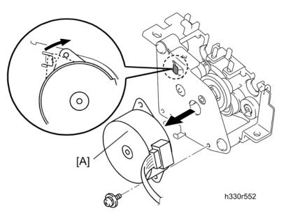
28. Remove the scanning motor F sub ASSY [A] (  $\mathscr{F}$  x 1; M3x6).
