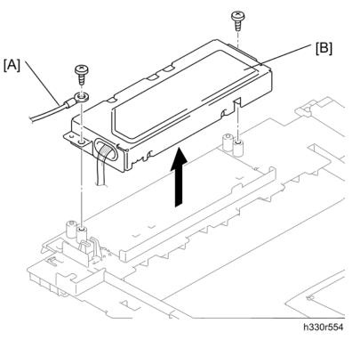
3. Remove the scanning drive LF FG harness [A] and NCU unit [B] (  $\Re$  x 2; B M4x12).
