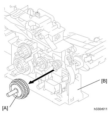
2. Remove the gear ASSY [A] from the main frame  $L\left[ B\right] .$
