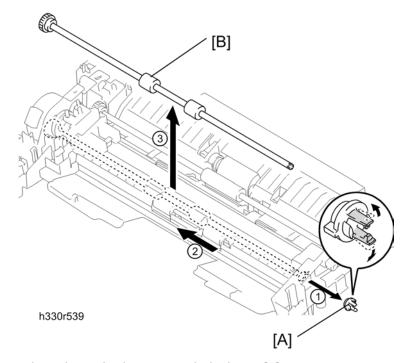
12. Release the two hooks to remove the bushing  $5\ [A]$ .
