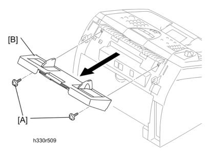
4. Remove the two screws (cup B M4x12) [A] to remove the document base ASSY [B].
