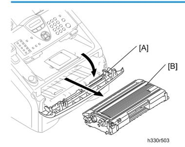
1. Open the front cover [A] and remove the drum/toner ASSY [B].
