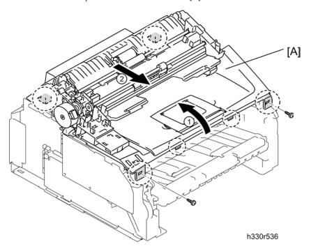
9. Release the six hooks to remove the top cover [A] (  $\mathscr{F}$  x 2; B M4x12).
