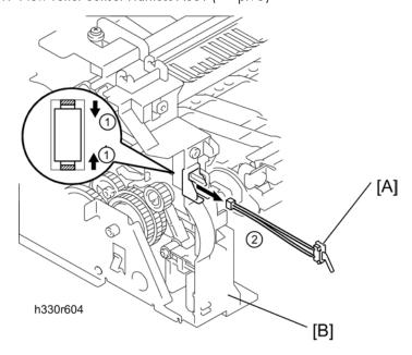
2. Release the two hooks and remove the cover sensor [A] from the main frame L [B].
