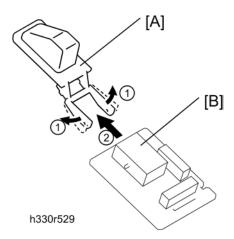
4. Remove the actuator hook [A] from the hook PCB ASSY [B].
