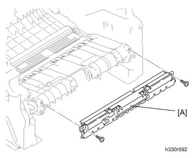
2. Remove the sub chute ASSY [A] ( $\mathscr{F}$  x 2; B M4x12).
