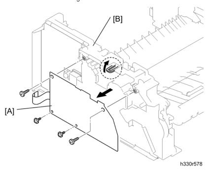
Remove the high-voltage PS PCB [A] from main frame L [B]. (Top ₹ x 2; B M4x12, Bottom ₹ x 2; S M3x6, hook)
