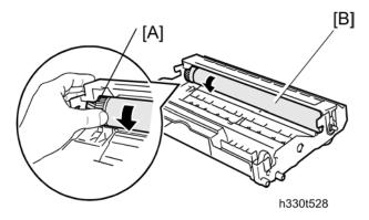
2. Turn the drum gear [A] by hand while looking at the surface of the exposure drum [B].
