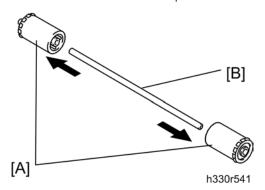
15. Remove the two pressure rollers [A] from the pressure roller shaft [B].
