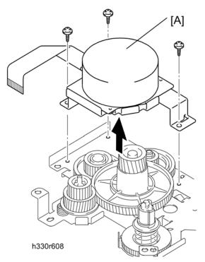
6. Remove the main motor ASSY [A] (  $\ensuremath{\mathcal{P}}$  x 3; S M3x6).
