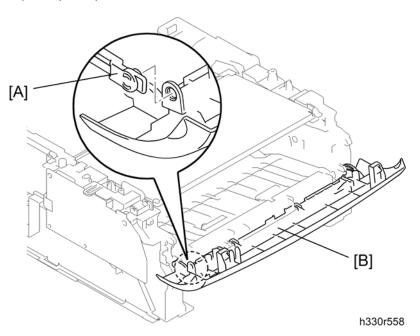
4. Release the hook [A] of the drive release cam from the front cover ASSY [B].
