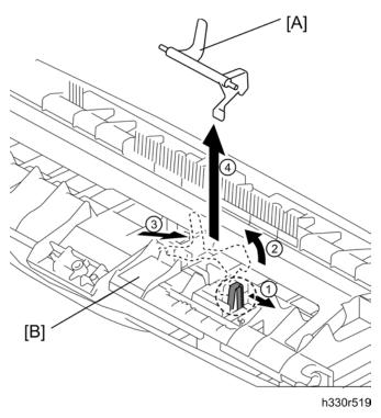
5. Remove the actuator R [A] from the panel unit [B].
