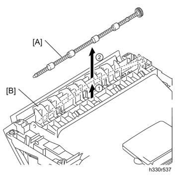
10. Remove the paper eject roller ASSY [A] from the top cover [B].
