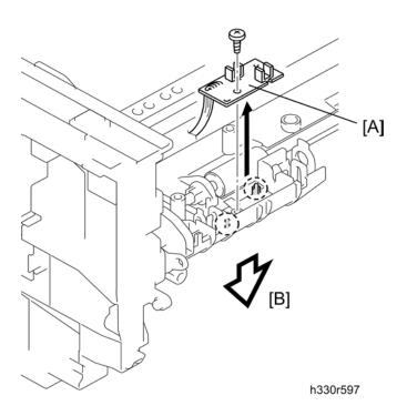
2. Release the harness from the hook and remove the regist sensor PCB ASSY [A] ( $\mathscr{F}$  x 1; B M3x6).
