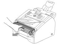
Hold down the lock lever on the left and pull the toner cartridge out of the drum unit. Take out the jammed paper if there is any inside the drum unit.
