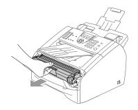
2 Clean the primary corona wire inside the drum unit by gently sliding the blue tab from right to left several times.
