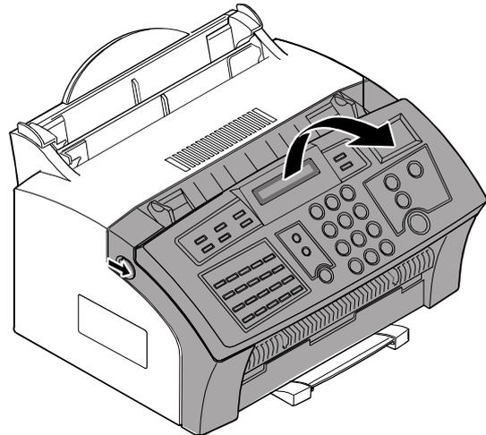
2. Remove the two stoppers holding the front cover unit and unplug one connector and one wire.
