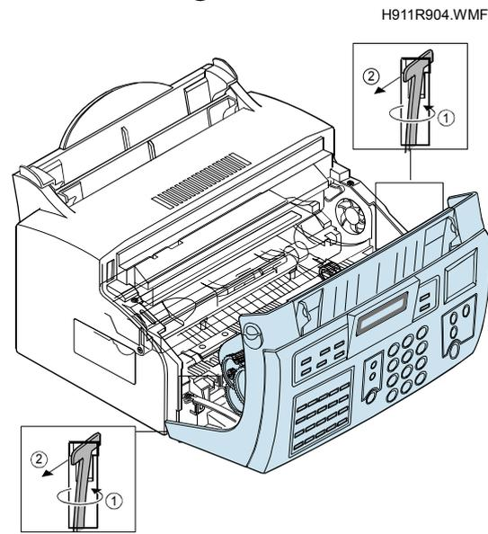
3. Pull the bottom left end of the cover downward to unlatch the front cover unit and remove the cover from the main frame.
