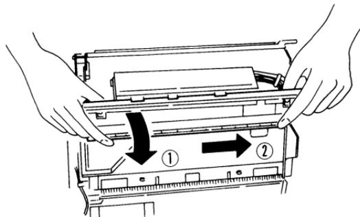
4. Check that the head is positioned properly and that the springs pushing the head against the platen roller are in position.
