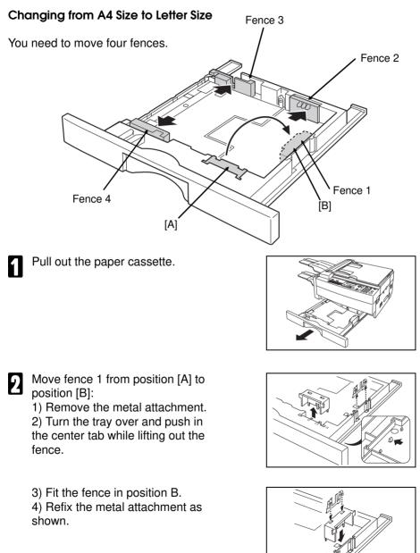
B Move fence 2 out a notch. Push in the center tab underneath while pushing in the other tab on top and lift out the fence.
