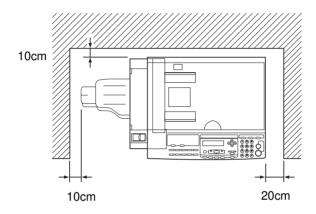
NOTE: This machine generates a certain amount of ozone. Although the amount generated is within safety requirements, it is recommended that, to avoid ozone buildup, you install the machine in a room which is properly ventilated.
