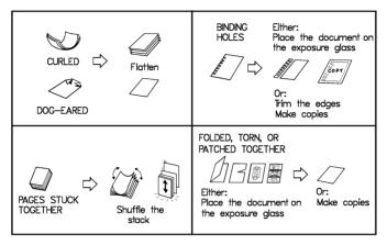
Originals that contain the following materials should not be placed in the document feeder. Place them directly on the exposure glass.
