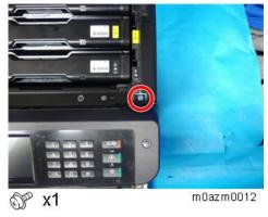
5. Standing at the front of the machine, pull and slide the operation panel toward you so it turns over, remove the 1 connector and 2 FFCs at the left side, and then remove the operation panel.
