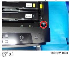
$\underline{\mathbf{5}}$ . Disconnect the harness on the back of the operation panel ( $\mathbf{5}$  x 1).
