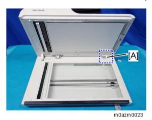
With the SP C262SFNw, replace the DADF unit and scanner unit together as the DADF/Scanner Assembly. For details about how to replace them, see DADF/Scanner Assembly.
