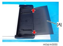
Open the DADF cover, disengage the hooks on the sides of the original tray [A], and then remove the tray.
