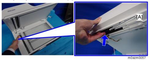
**2.** Cover the scanner exposure glass with a mat or something to prevent it from being damaged.
