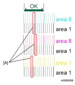
Four sets of vertical lines appear on the test chart (C and k, M and k, Y and k...). In each set, look for vertical lines that are aligned within the region defined by "OK".
