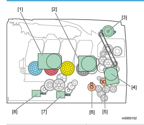
1. Color AIO Motor5. Registration Clutch2. Black AIO Motor6. Paper Feed Clutch3. Duplex Motor7. Agitator Motor4. Transport/Fusing Motor8. ITB (Image Transfer Belt) Contact Motor
