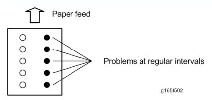
Image problems may appear at regular intervals that depend on the circumference of certain components. The following diagram shows the possible symptoms (black or white dots at regular intervals).
