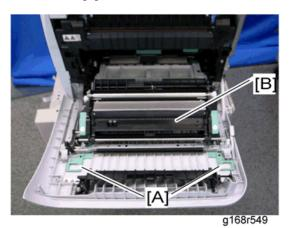
4. If you install a complete new unit, execute "Reset 2nd Transfer Unit" with the "Engine Maintenance" menu (page 130 "Maintenance Mode Menu (MF Models)" or page 142 "Service Mode (Printer Models)").
