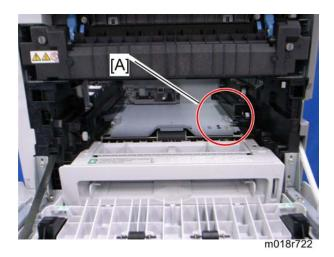
8. Clean inside the printer, especially around the circled area [A].
