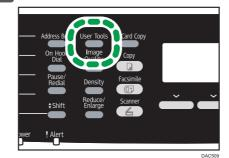
Press the [▼] or [▲] key to select [Network Settings], and then press the [OK] key.
