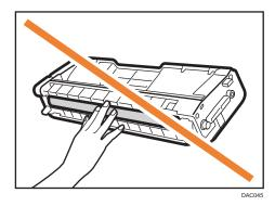
• Do not touch the ID chip on the side of the print cartridge as shown below.
