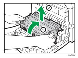
4. Holding the handle at the center of the waste toner bottle, carefully pull it partially out without tilting it.
