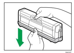
6. Check the toner color and corresponding location, and then carefully insert the print cartridge vertically.
