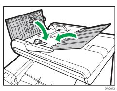
4. Lift the ADF, and if there is any original remaining in the ADF, gently pull the jammed paper to remove it.
