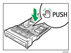
6. Reload the removed paper into the tray, and then push the tray carefully into the machine until it clicks.
