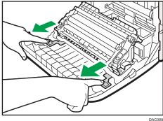
3. Holding the tabs on both ends of the transfer unit, tilt it backwards and lift it up.
