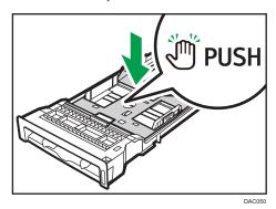
4. Pinch the extender in the "PUSH" direction, and then pull out the extender until it clicks.
