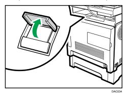
• Pull up the retainer as shown below to prevent Legal-size printed copies from falling off.
