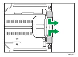
After extension, check that the arrows on the extender and tray are aligned.
