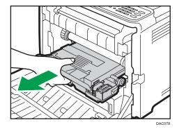
To prevent the waste toner bottle from coming into contact with the intermediate transfer unit (the position shown by the arrow in the illustration below), do not lift the bottle while pulling it out.
