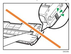
• When removing print cartridges, be careful not to touch the laser scanning unit under the upper cover (the position shown by the arrow in the illustration below).
