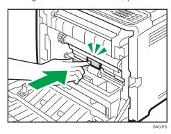
9. Place the transfer unit on the front cover. Slide the transfer unit along the guide rails into the machine.
