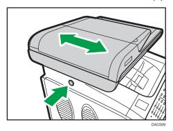
• Pull up the retainer as shown below to prevent A4- or Letter-size printed copies from falling off.
