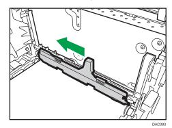
4. Carefully insert the print cartridge removed in Step 2 vertically.
