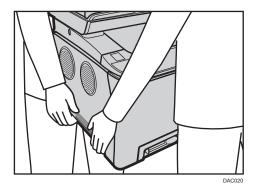
5. There are three upright pins on the optional paper feed unit. Align them with the holes on the underside of the machine, and then carefully lower the machine.
