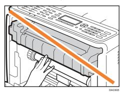
If paper has jammed inside the transfer unit, holding both sides of the paper, pull the paper carefully forward and out.
