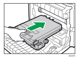
To prevent the waste toner bottle from coming into contact with the intermediate transfer unit (the position shown by the arrow in the illustration below), do not lift the bottle while inserting it.
