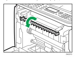
3. Pull up the fusing unit levers.
