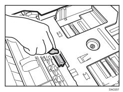
5. Wipe the rubber part of the roller with a soft damp cloth. After that, wipe it with a dry cloth to remove the moisture.
