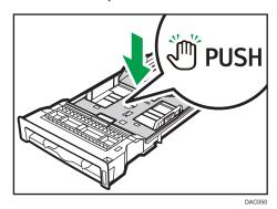
7. Reload the removed paper into the tray, and then push the tray carefully into the machine until it clicks.
