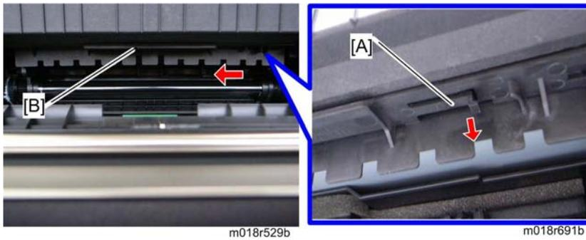
5. Release the hook [A] under the guide plate.
