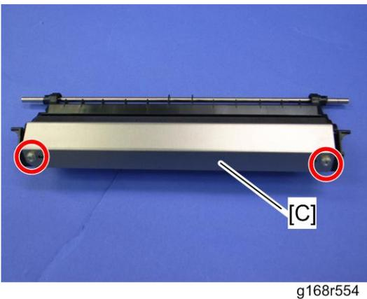
4. Transfer roller assembly [C] (
