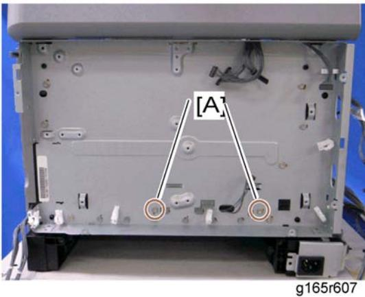
4. Remove two screws [A] for the waste toner sensor base.
