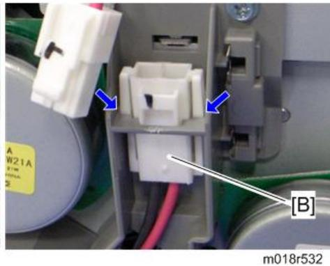
2. Disconnect the fusing connector [A] and remove the fusing relay harness [B] (hooks x 2).
