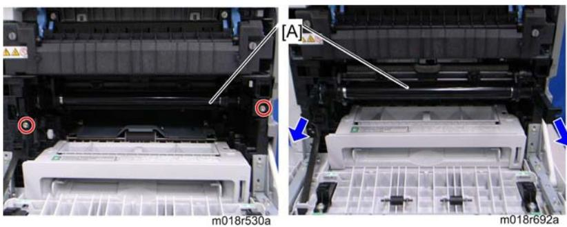
7. Pull out the image transfer belt unit [A] (
