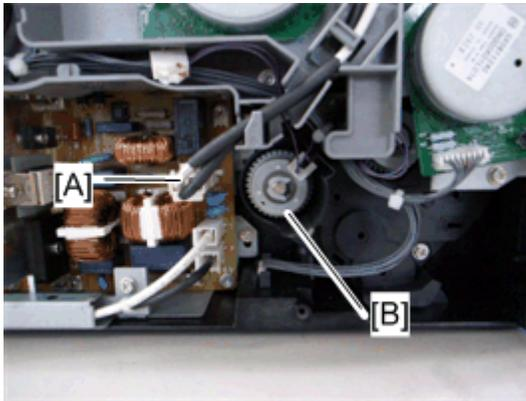
3. Disconnect the fusing relay harness [A] (hook).
