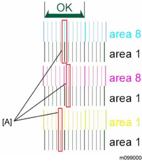
Four sets of vertical lines appear on the test chart (C and k, M and k, Y and k...). In each set, look for vertical lines that are aligned within the region defined by "OK".
