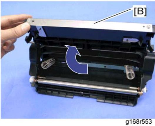
3. Open the transfer roller unit [B] and remove it.
