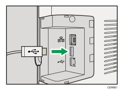
When the printer recognizes the digital camera as a PictBridge device, "PictBridge Connecting...", then "Ready" will appear on the printer's control panel.
