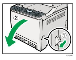
7. Pull the opening lever on the front cover, and then carefully lower the front cover.
