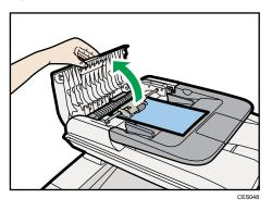
5. Move the lever slightly to the machine rear, and then pull it up to unlock the paper feed roller.
