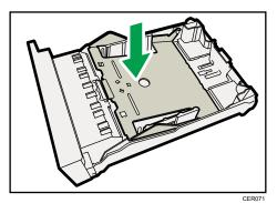
3. Pinch the clips on the side paper guide, and then adjust the guide to the paper size.
