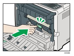
9. Place the transfer unit down on the front cover.
