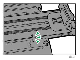
5. Pinch the clip on the side paper guide, and then slide it to match the paper size.
