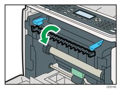
3. Pull up the fusing unit levers.
