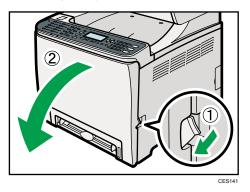
1. Pull the opening lever on the front cover, and then carefully lower the front cover.
