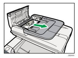
3. If you cannot pull out the jammed original easily, move the lever slightly to the machine rear, and then pull it up to unlock the paper feed roller.
