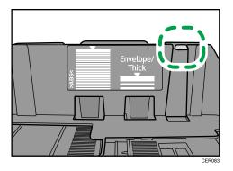
6. Check there are no gaps between the paper and the paper guides; both side and front end paper guides.
