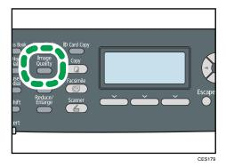
2. Press the [▲][▼] keys to select the desired resolution setting, and then press the [OK] key.
