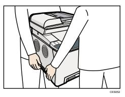
5. There are three upright pins on the optional paper feed unit. Align them with the holes on the underside of the machine, and then carefully lower the machine onto them.
