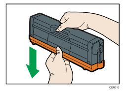
6. Check the toner color and corresponding location, and then carefully insert the print cartridge vertically.
