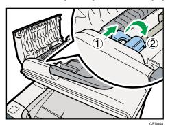
4. Lift the paper feed roller slightly and pull it out toward you.
