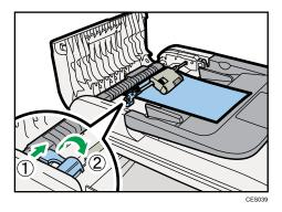
6. Lift the paper feed roller slightly to remove it.
