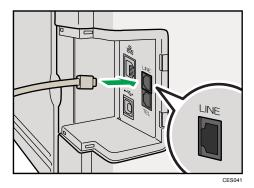
3. If using an external telephone, connect the telephone to TEL.
