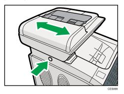
• Pull up the fence as shown below to prevent A4- or Letter-size prints from falling off.
