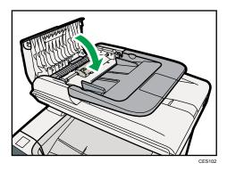
11. Lift the ADF, and if there is original remaining in the ADF, gently pull the jammed original to remove it.
