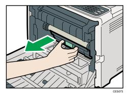
5. Pull the waste toner bottle halfway out, grab the bottle firmly, and then pull it straight out.
