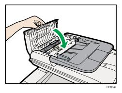
12. Pull the opening lever on the front cover, and then carefully lower the front cover.
