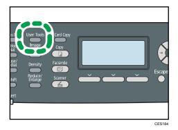
2. Press the [<sup>A</sup>][<sup>V</sup>] keys to select the file you want to delete, and then press the [OK] key.
