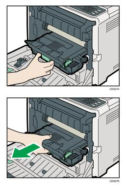
To prevent the waste toner bottle touching the intermediate transfer unit (the position shown by the arrow in the illustration below), do not lift the bottle while pulling it out.
