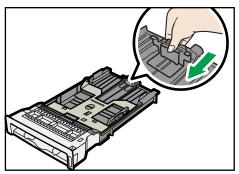
4. Pinch the front end paper guide and slide it inward to match the standard size.
