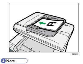
• When placing originals longer than A4, pull out the ADF tray's extenders.
