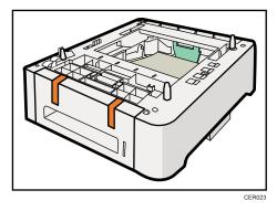
4. Lift using the inset grips on both sides of the machine.
