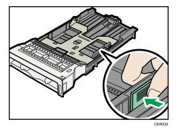
5. Pinch the clip on the front end paper guide to match the envelope size.
