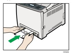
After the envelope is inserted until it stops, the envelope will be automatically fed into the machine a little.
