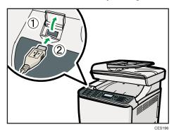
When the machine recognizes the digital camera as a PictBridge device, "PictBridge Connecting...", then "Ready" will appear on the machine's control panel.
