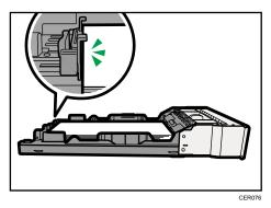
If there is a gap between the paper and the front end paper guide, as in the example below, the paper might not feed in correctly.
