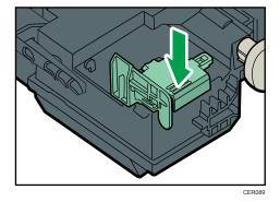
7. Hold the center of the new waste toner bottle, and then carefully insert it halfway into the machine body.
