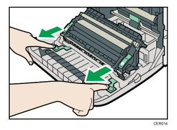
3. Holding the tabs on both ends of the transfer unit, tilt it backwards then lift it up.
