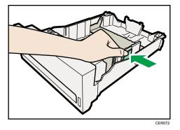
4. Pinch the clip on the end paper guide and align the arrow with the paper size.
