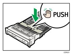
4. Pinch the extender in the "PUSH" direction, and then pull out the extender until it stops (you will hear a click).
