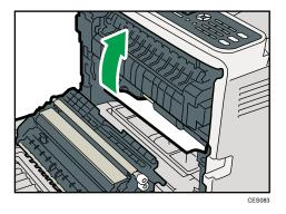
If paper has jammed inside the transfer unit, holding both sides of the paper, pull the paper carefully forward and out.
