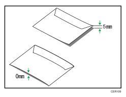
• If the curl is severe, flatten out the envelopes using your fingers, as shown in the illustration below.
