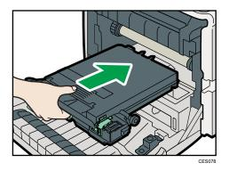
To prevent the waste toner bottle touching the intermediate transfer unit (the position shown by the arrow in the illustration below), do not lift the bottle while inserting it.
