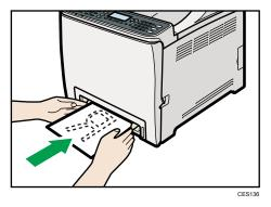
After the paper is inserted until it stops, the paper will be automatically fed into the machine a little.
