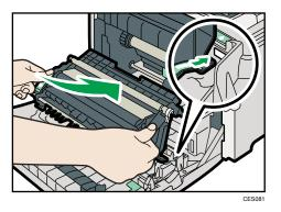
10. Slide the transfer unit along the guide rails into the machine. When it stops, push on the PUSH mark until it clicks into place.
