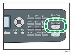
6. Press [TX], and then press the [B&W Start] key.
