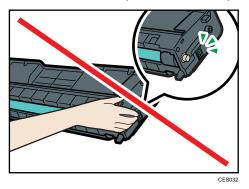
• When removing print cartridges, be careful not to touch the Laser Scanning Unit on the underside of the upper cover (the position shown by the arrow in the illustration below).
