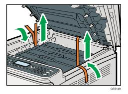
18. Lift out print cartridges and shake them from side to side. The black print cartridge comes with a protection sheet that you must remove before shaking.
