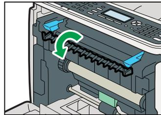
**4** Pull up the fusing unit levers.
