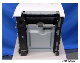
8. Stand the printer with the rear side facing the table.
