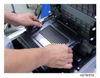
12. Remove the laser optics housing unit.
