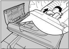
4 Lift the paper feed roller slightly and pull it out toward you.
