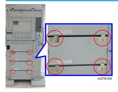
1. Attach the six brackets and six screws as shown above.
