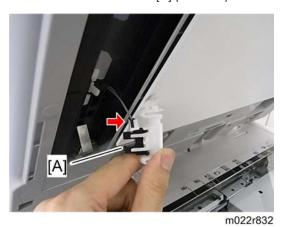
4. ARDF inverter sensor (🗂 x 1, hooks)
