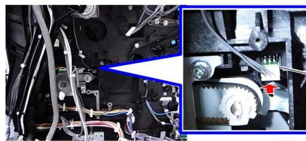
3. Duplex relay sensor [A] (hooks, 📬 x 1)
