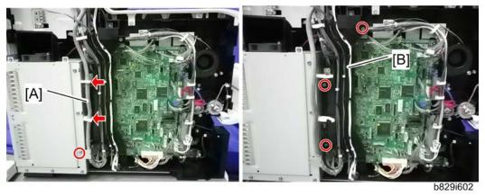
3. Take aside the scanner I/F cable [A] (  $\mbox{\ensuremath{\not\sim}} \times 1$  ,  $\mbox{\ensuremath{\ensuremath{\bowtie}}} \times 2$  ).
