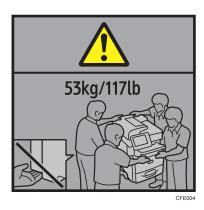
Type 3 weighs approximately 52 kg (114.7 lb.). When moving the machine, use the inset grips on both sides. At least four people are needed to lift the machine.
