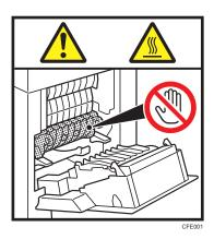
The inside of this machine becomes very hot. Do not touch parts with this label (indicating a hot surface).
