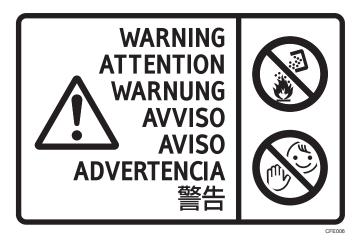
Do not incinerate spilled toner or used toner. Toner dust is flammable and might ignite when exposed to an open flame.
