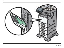
2. Insert the paper face up until you hear the beep, and then align the paper guides to the paper size.
