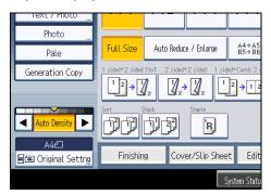
6. Place the originals in the orientation displayed in "Original Setting", and then press the [Start] key.
