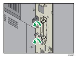
5. Fully insert the Gigabit Ethernet board.
