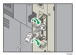
8. Attach the antennas of the wireless LAN with the hook and loop fasteners that you attached in step 3, and then place the cables in the cable clamps and close the clamps.
