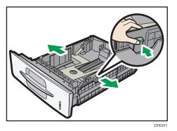
3. While pressing down the release lever, slide the end fence until it is aligned with the size of paper you want to load.
