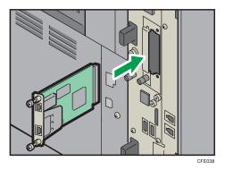
**6.** Tighten two screws to secure the Gigabit Ethernet board.
