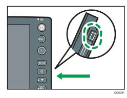
When it is inserted correctly, the media access lamp beside the media slot lights.
