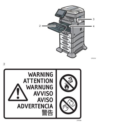
Do not incinerate spilled toner or used toner. Toner dust is flammable and might ignite when exposed to an open flame.
