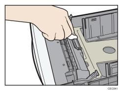
6. Wipe the rubber part of the roller with a soft damp cloth. After that, wipe it with a dry cloth to remove the moisture.
