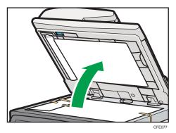
10. Remove the protective material attached on the exposure glass.
