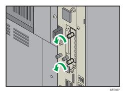
5. Fully insert the Gigabit Ethernet board.
