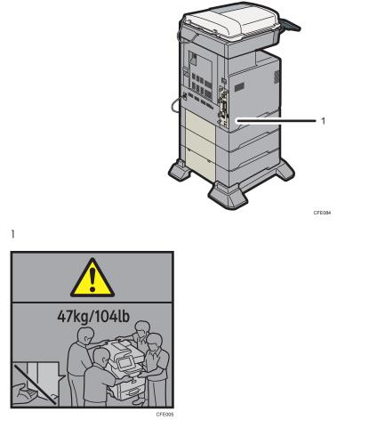
Type 1 weighs approximately 45 kg (99.2 lb.) and type 2 weighs approximately 47 kg (103.7 lb.). When moving the machine, use the inset grips on both sides. At least four people are needed to lift the machine.
