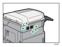
4. Remove the seals from the cable clamps, and then attach them to the left side of the machine.
