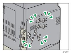
5. Loosen two screws and remove the cover of the slot in which the wireless LAN interface board is installed.
