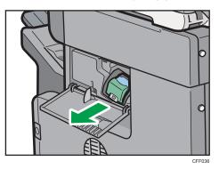
3. Hold both sides of the empty refill, pull up, and remove it.
