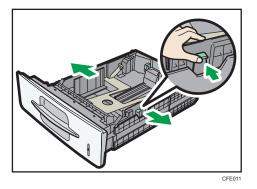
4. While pressing down the release lever, slide the end fence until it is aligned with the size of paper you want to load.
