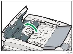
3. Wipe the paper pickup roller, paper feed roller, and friction pad with a soft damp cloth. After that, wipe them with a dry cloth to remove the moisture.
