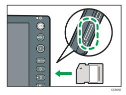
When it is inserted correctly, the media access lamp beside the media slot lights.
