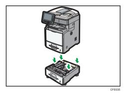
When installing two or more units, first connect the units together, and then attach them as a single unit to the machine.
