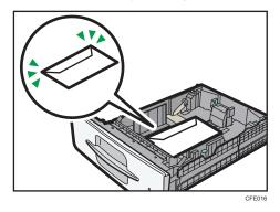
• When loading envelopes in trays 1 <sup>-</sup> 4 or the bypass tray, open the rear cover, and then raise the envelope lever.
