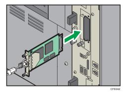
7. Tighten two screws to secure the interface board.
