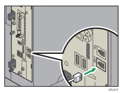
2. If using an external telephone, connect the telephone to the external telephone connector (TEL).
