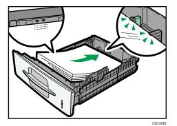
4. Hold the tray with both hands, slide it along the rails of the machine, and then push it straight in.
