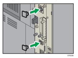
4. Loosen two screws and remove the cover of the slot in which the Gigabit Ethernet board is installed.
