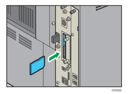
Insert the SD card in the lower slot.
