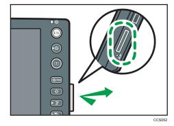
3. Pinch the SD card, and then pull it carefully out of the slot.
