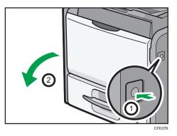
13. Hold the print cartridge's front handle to lift and pull it out.
