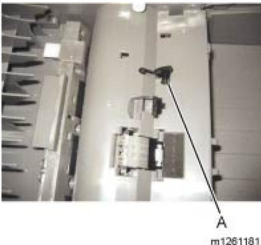
3. To test the paper present sensor, push back on the actuator (A). If the sensor is functioning, the 0 next to the P on the display will change to 1.
