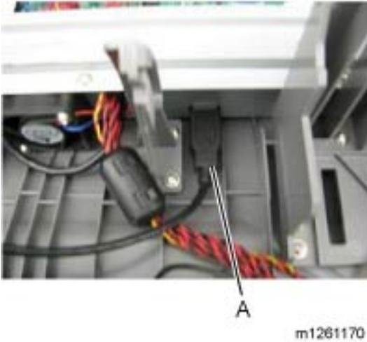
4. Disconnect the card reader cable (A) from the J2 USB port on the controller board.
