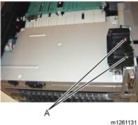
4. Remove the two screws (A) from the right rear foot assembly.
