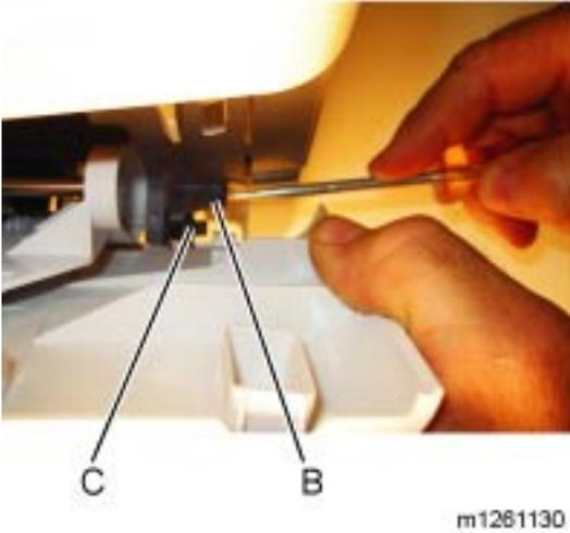
**Installation note:** Use a flathead screw driver to press in on the door mount (B) while pulling on the front access door to connect the cover to the hinge (C).
