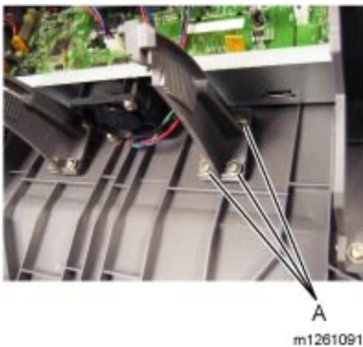
2. Remove the three screws (A) securing the display rotation support to the tub assembly.
