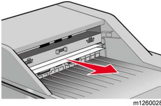
2. Pull out the jammed media by pulling on the bottom sheet.
