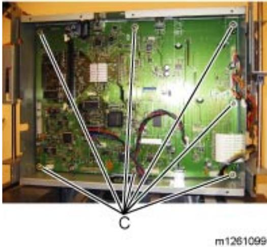
5. Remove the seven screws (C) securing the controller board to the controller board cage.
