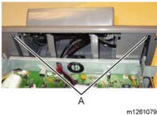
4. Release the two tabs (A) securing the keypad to the keypad to the tub assembly.
