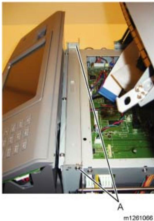
1. Remove the two screws (A) securing the controller shield bracket to the controller board cage.
