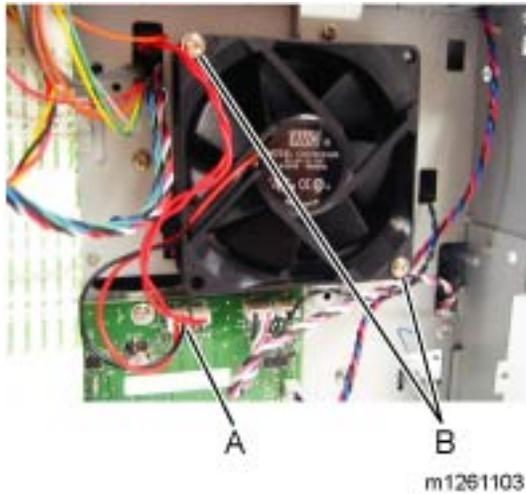
2. Disconnect the cable (A) from the engine board, and remove the two screws (B) holding the fan to the right side frame.
