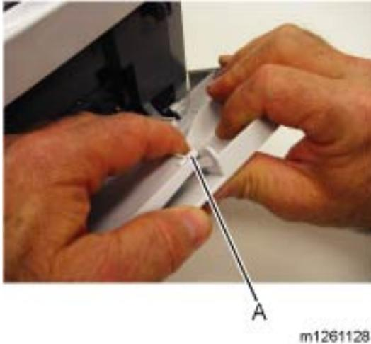
2. Disconnect the MPF pins (A) from the right and left sides of the lower front cover.
