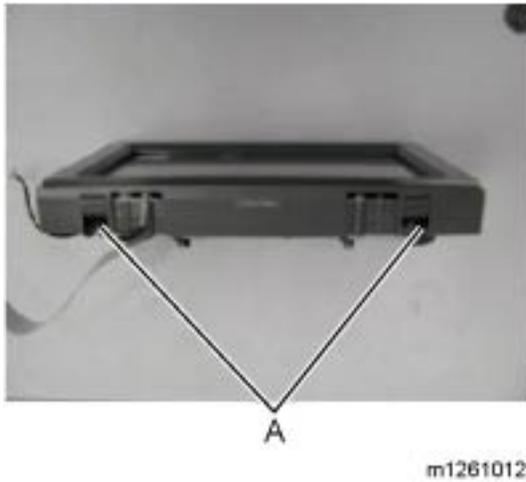
2. Depress the two tabs (A) securing the display bezel to the operator panel display.
