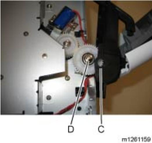
6. Disconnect the left hinge (C) from the feed clutch, and remove the e-clip (D).
