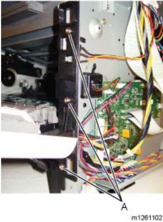
6. Remove the three screws (A) from the right side of the printer.
