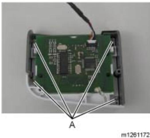
3. Remove the four screws (A) fastening the upper and lower card reader covers.
