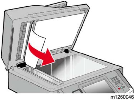
1. Lift the flatbed cover, and remove the jammed media from the ADF.
