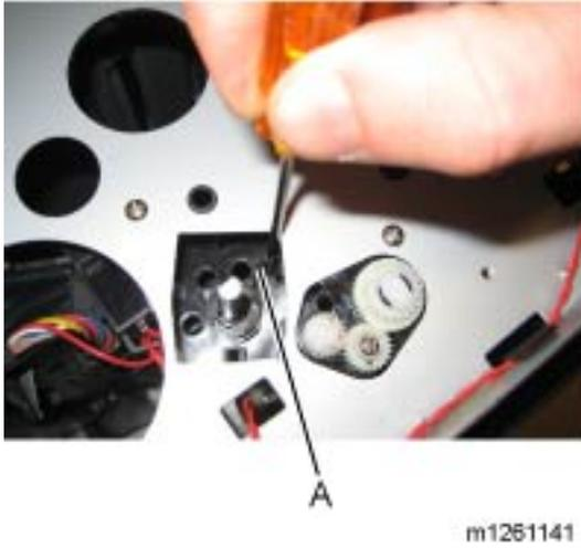
6. Use a screwdriver to pop the shaft retainer tab (A) loose from the ACM feed shaft.
