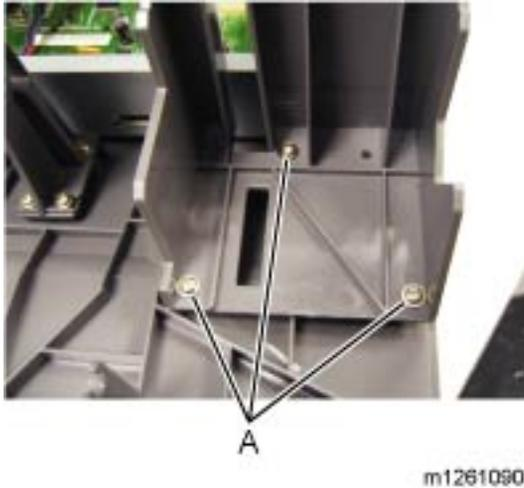
2. Remove the three screws (A) securing the operator panel support to the tub assembly.
