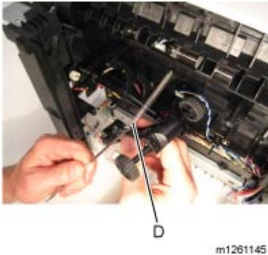
10. Pull out the auto compensator shaft, and remove the spring (D).
