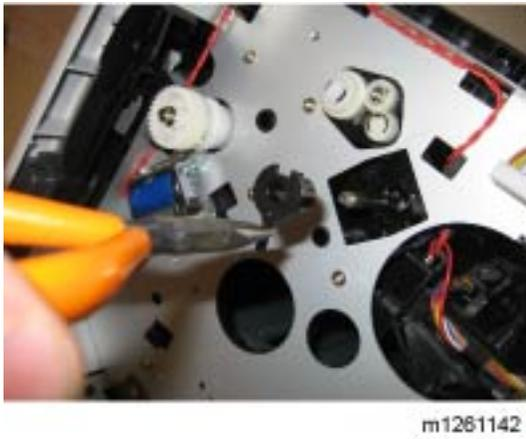
7. Use a small pair of pliers to remove the shaft retainer tab.
