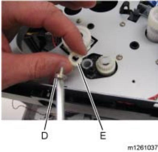
6. Remove the screw (D) from the gear (E).
