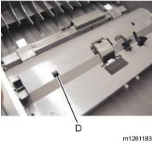
7. To test the ADF cover open sensor, open the ADF top cover. If the sensor is functioning properly the 0 next to the A will change to 1.
