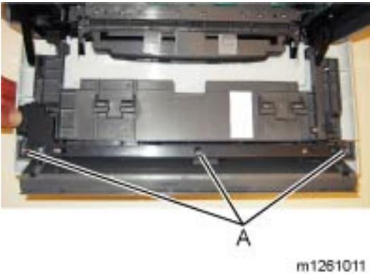
2. Remove the three screws (A).
