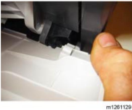
3. Flex the lower front cover, and disconnect it first from its right hinge and then from its left hinge.
