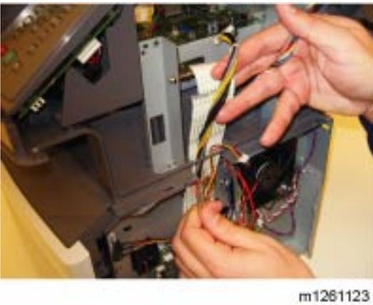
11. Thread the LSU diode cable, the cover interlock cable, the stairway cables, and the controller board power supply cable through the side of the printer away from the scanner assembly.
