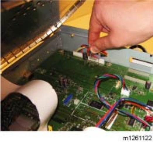
10. Disconnect the LSU laser diode cable from the controller board.
