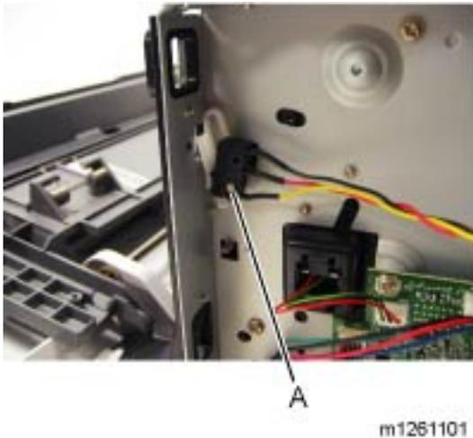
3. Remove the screw (A) holding the sensor.
