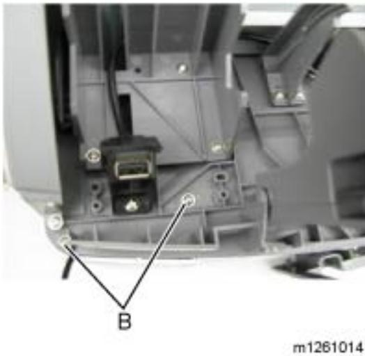
5. Remove the two screws (B) securing the card reader housing to the tub assembly.
