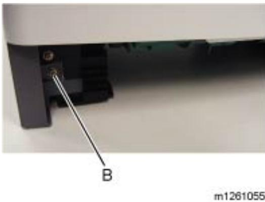
4. Remove the metal screw (B) that secures the left cover to the front of the print engine frame.
