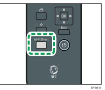
The LED of the [Wi-Fi Direct] key starts flashing.
