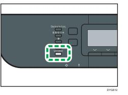
The LED of the [Wi-Fi Direct] key starts flashing.
